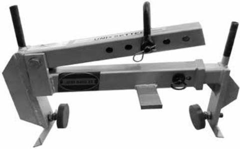
The UNISSETTER is a tool that is easily adjusted to fit a wide variety of man-made as well as natural stones, steps or stair treads. The lifting method is from the face to the back of the stair tread, thus allowing the versatility of setting them between walls. The UNISSETTER will adjust from 13" to 25" with the standard arm.
